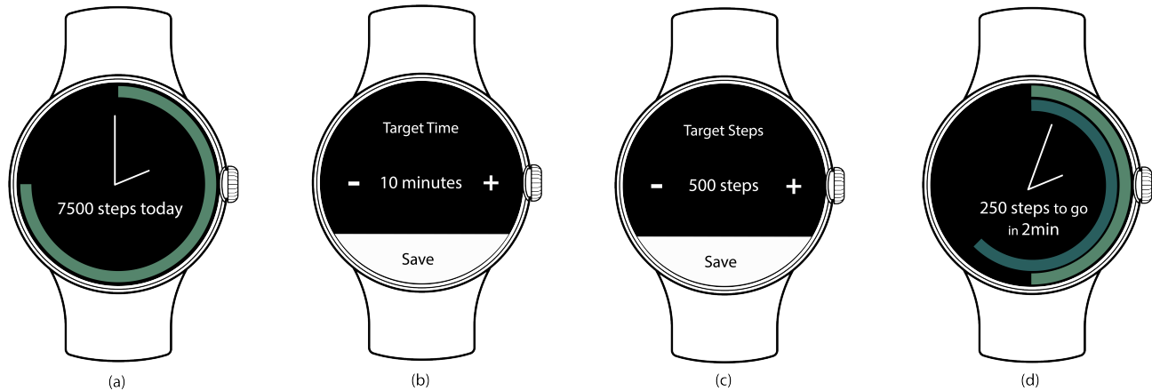
Figure 1: Users create a micro-goal by double-tapping the smartwatch screen. They start by setting the target duration (b) and number of steps (c) for the micro-goal. Mikro then displays users’ micro-goal progress through two rings (d): the outer ring represents step count progress - filling up as steps were accumulated towards the target, while the inner ring shows elapsed time. When no micro-goal is active, Mikro displays feedback on progress towards a daily step count goal (a).
