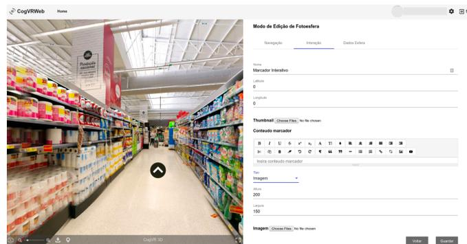
Fig. 2. Enriching an environment. The environments can be enriched for instance with interactive images or transparent areas that trigger a sound or a message; or with HTML content to guide the user during navigation. At the left side of the screen the users may see the environment and click to define the position of the interaction points. At the right side the users may for instance add interactions to a photo sphere or define the navigation paths.
