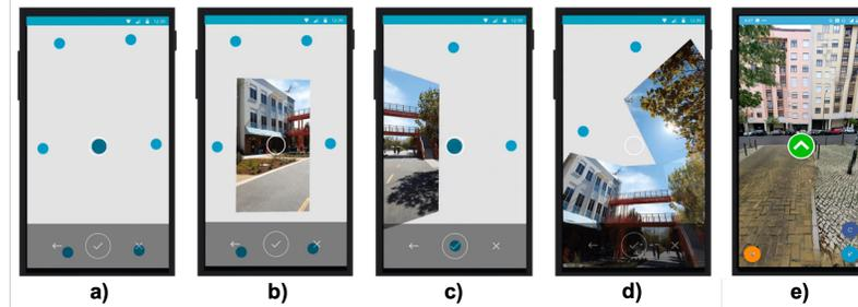
Fig. 1. To capture a 360° photo: a) point the center of the screen over one of the various existing circles, keeping the smartphone fixed until the captured photograph appears; and b), c) and d) repeat this process until there are no more circles or users are satisfied (users may capture only the parts that they want, i.e. they can ignore the back part or the ceiling). After taking a photo sphere, e) the users are able to select all positions where new photo spheres will be linked.
