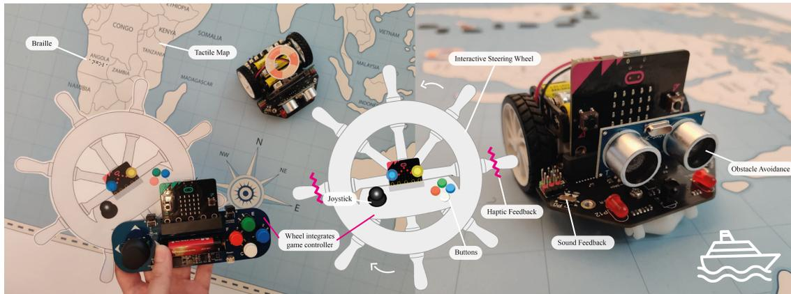
Fig. 1. TACTOPI, a playful environment designed from the ground up to be rich in both its story (a nautical game) and its mechanics (e.g., a physical robot-boat controlled with a 3D printed wheel), tailored to promote computational thinking at different levels (4 to 8 years old).
